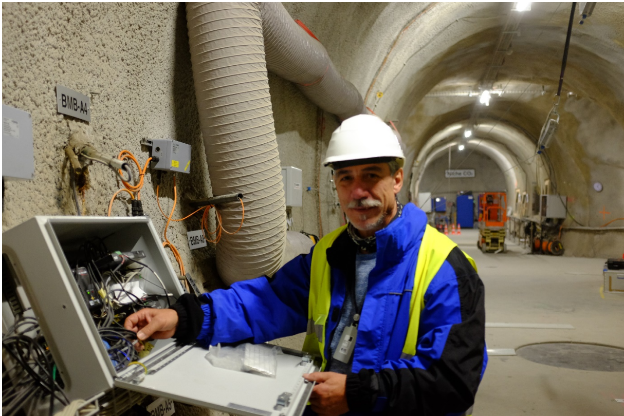
Figure 1: SW-A: F. Königer is checking the connection of the Taupe sensors (Photo: S. Schefer, swisstopo).
