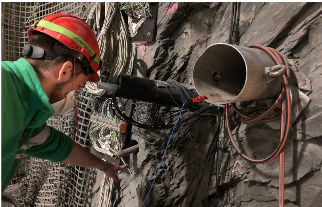
Figure 2: PF: M. Felder changing the grounding cable from a packer to the steel casing to produce better results (Photo: S. Schefer, swisstopo).
