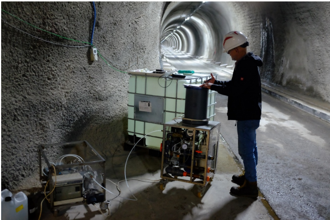
Figure 2: HS: Degassing and sampling for geochronology of pore water coming from interval 2 of BHS-1 (Photo: A. Degiacomi, swisstopo).
