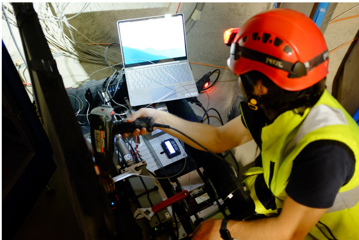
Figure 1: CS-E: A. Rinaldi heating the gas line for the miniRuedi to evaporate the water trapped inside (Photo: S. Schefer, swisstopo).
