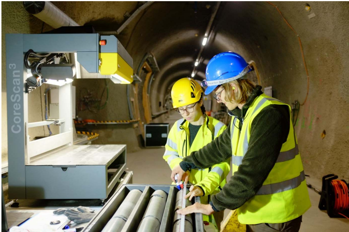
Figure 2: CS-D: M. Lukovic (I.) and Q. Wenning (ETHZ) preparing a drillcore for the CoreScan 3 core scanner. This new device of swisstopo is able to make high resolution core photos and HD 3D-models of any drillcore (Photo: S. Schefer, swisstopo).
