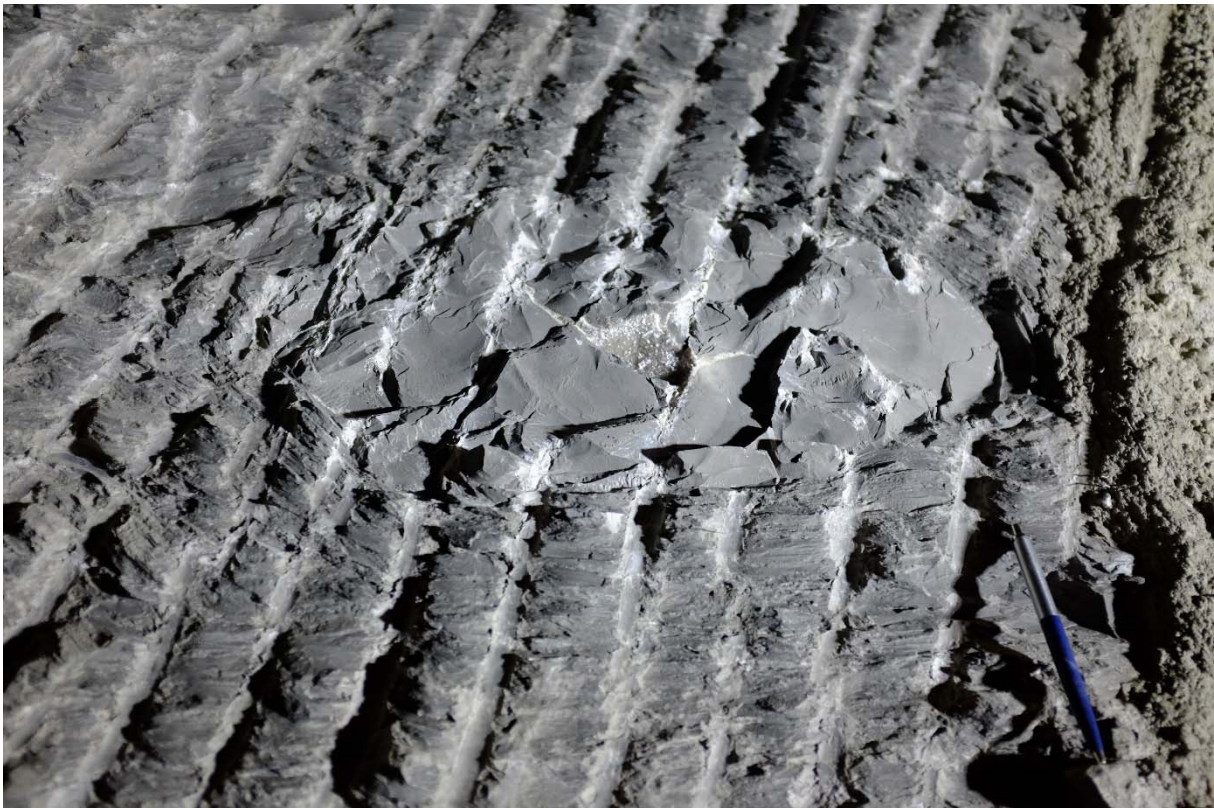
Figure 2: Ga18: Several calciferous nodules have been observed in the sandy facies of the OPA. This particular example has a diameter of almost 40 cm and shelters a hollow core filled with a calcite-crystal-crust similar to the interior of a geode (Photo: S. Schefer, swisstopo).
