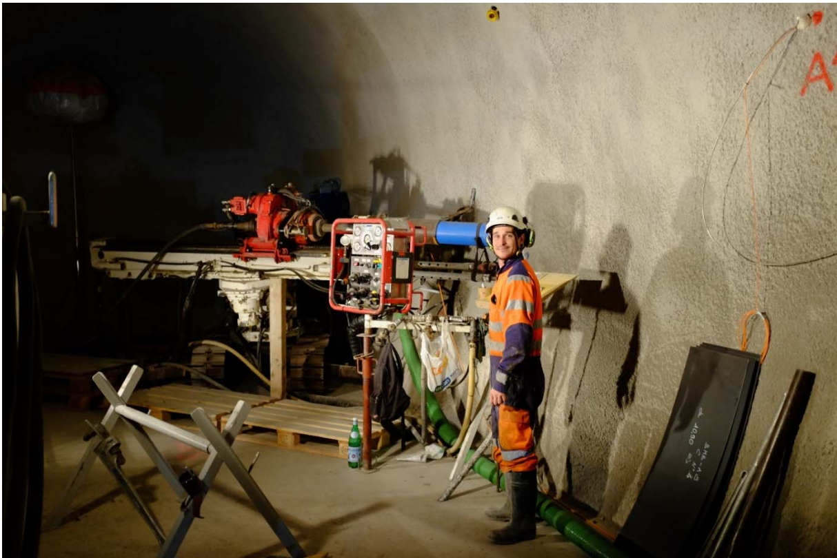
Figure 2: MB-A experiment: The drilling campaign continued. D. Gabin (GeoSonic) proceeding the drilling of borehole BMB-A8 (Photo: R. Raselli, swisstopo).
