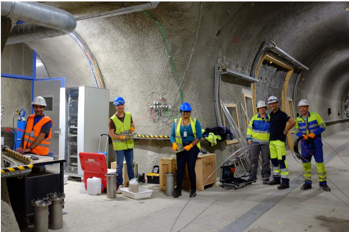
Figure 3: IC-A experiment: AMEC, EPFL, Nagra and Solexperts exchanged 6 of the IC-A modules (Photo: S. Schefer, swisstopo).
