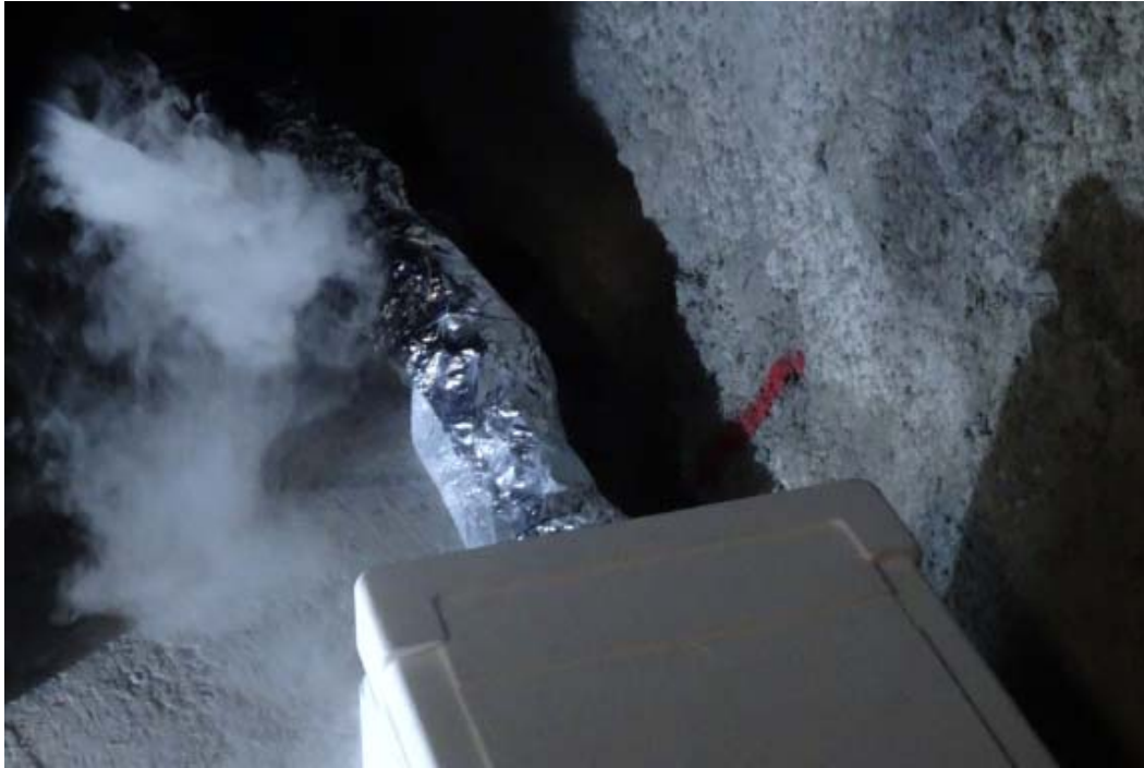
Figure 1: CI-D: The freezing of interval and packer lines in the HE-D Niche in preparation for the cutting of the lines (Photo: U. Mäder, University of Bern).
