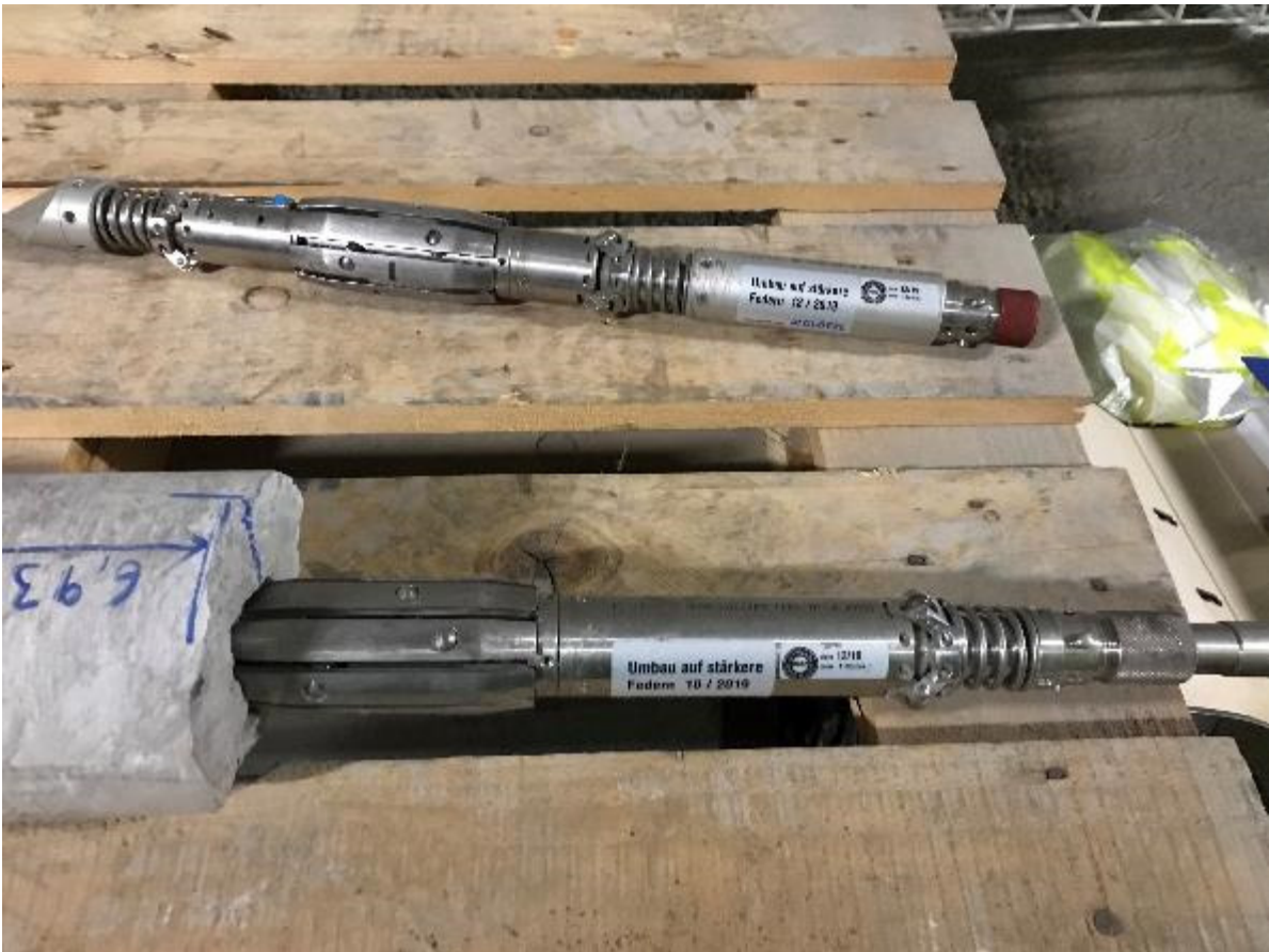
Figure 3: SW-A: Image of the hollow cylinder with the strain probes (Photo: D. Jaeggi, swisstopo)
