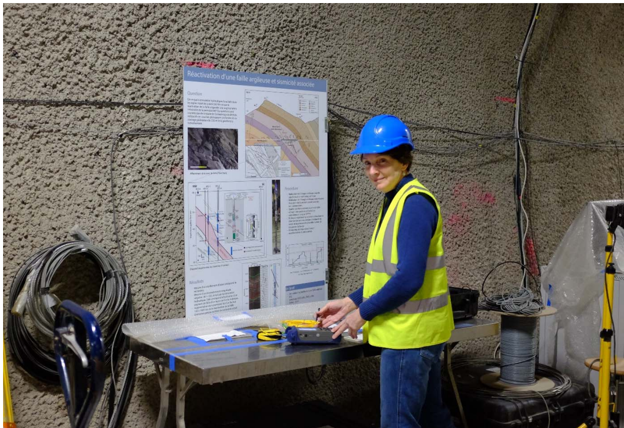
Figure 3: FS-B: M. Robertson (LBNL) measuring and controlling if the fiber optic cables installed behind casing in the five inclined geophysical boreholes BFS-B3 to BFS-B7 are working properly. They do. (Photo: R. Raselli, swisstopo).
