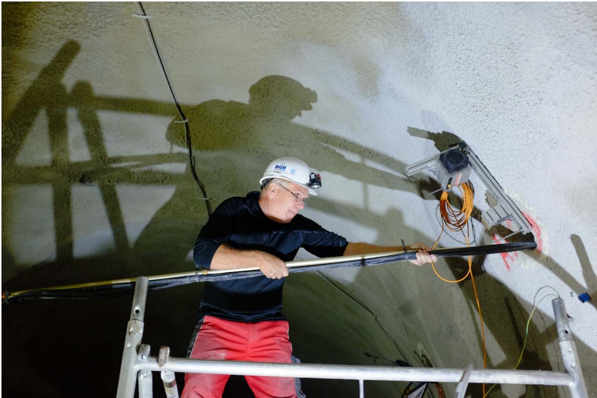
Figure 1: MB-A: F. Schulte (BGR) conducting interval velocity measurements (IVM) and electrical resistivity tomography (ERT) measurements (Photo: S. Schefer, swisstopo)
