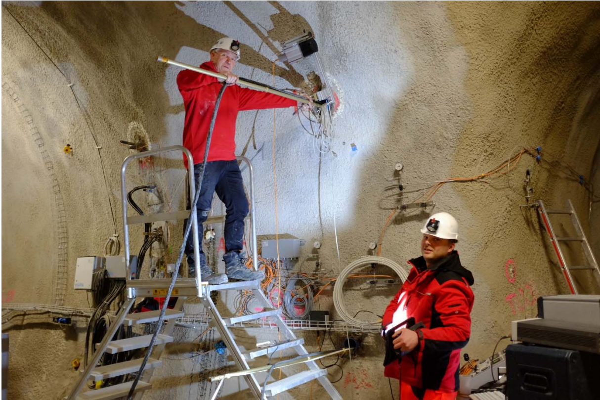
Figure 1: MB-A: F. Schulte and H. Albers (BGR) performing a cross-hole measurement (XHM) between BMB-A2 and BMB-A3 (Photo: J. Obrecht, swisstopo).
