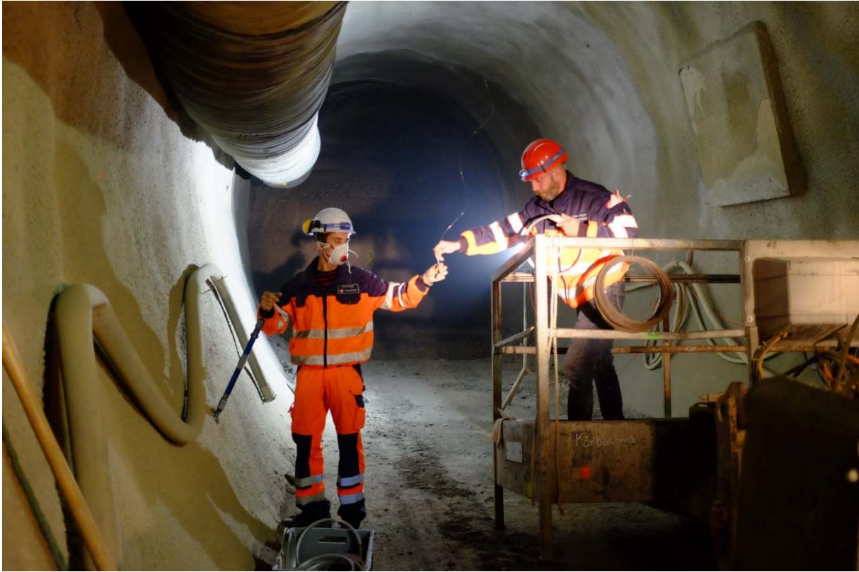
Figure 1: Ga18: D. Jaeggi and T. Theurillat (swisstopo) measuring convergences in Ga 18 (Photo: R. Raselli, swisstopo).
