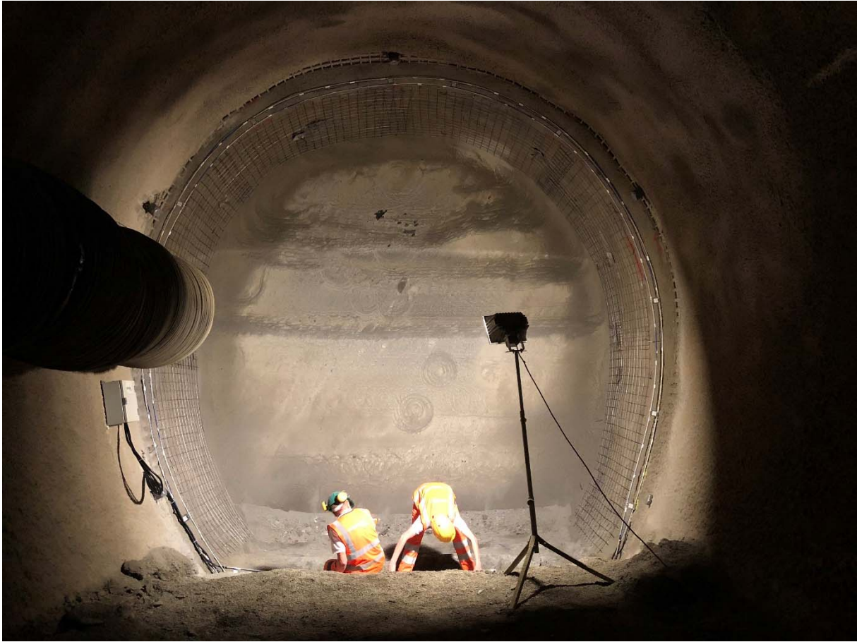
Figure 2: TS experiment: H. Zimmermann and A. Vlasek installing the first profile of fibre-optics in TS-1 (Photo: F. Fischli, Marmota Engineering AG).
