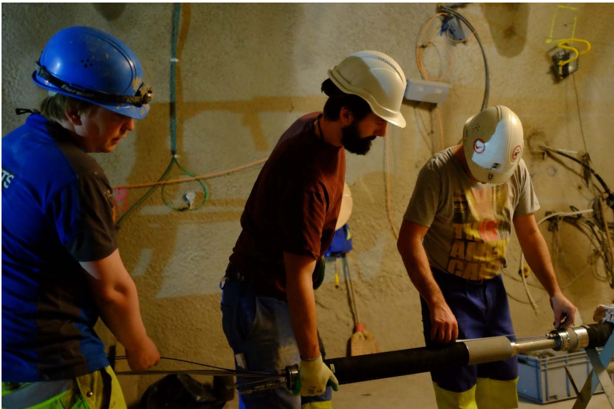
Figure 1: CS-D experiment: The team from Solexperts installing the packer system into BCS-D2 (Photo: S. Schefer, swisstopo)
