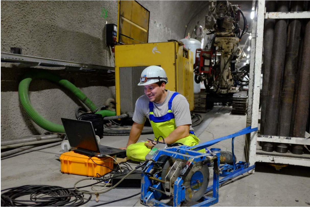
Figure 2: FS-B: D. Fischer (Terratec GmbH) performing an optical borehole imager (OBI) log (Photo: S. Schefer, swisstopo).
