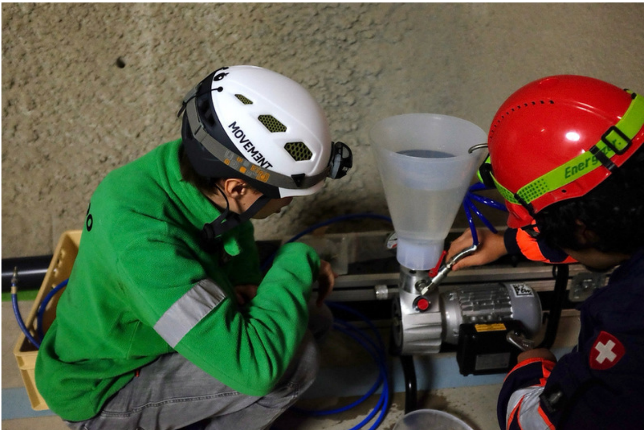
Figure 2: CL: J. Windisch and L. Borgeaud (swisstopo) testing the resin pump for CL experiment (A. Grignaschi, swisstopo).
