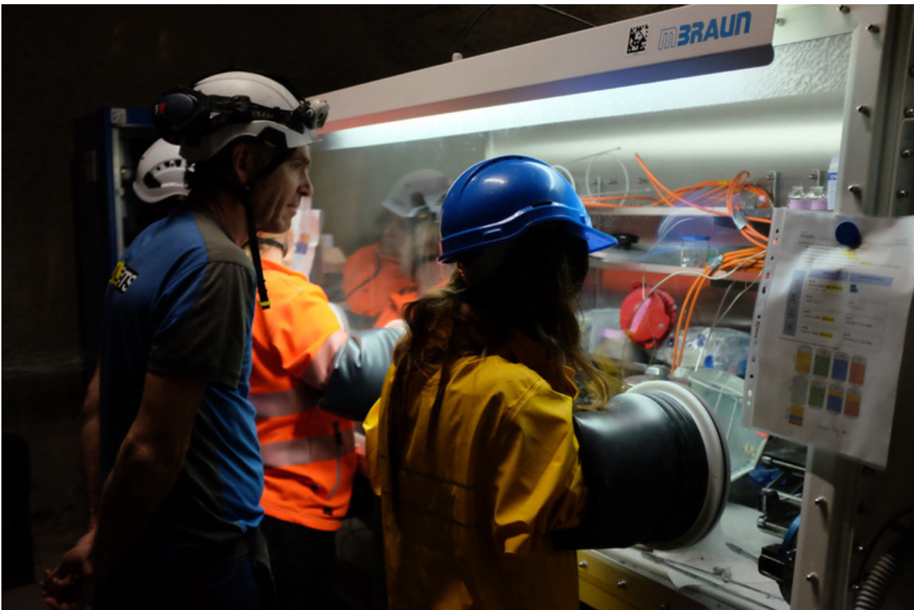
Figure 3: IC-A: Removing the samples in a controlled environment inside the glovebox (P. Steiner, swisstopo).
