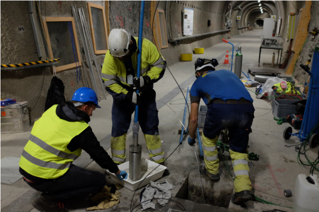
Figure 2: IC-A: The samples are below a packer and well stored (P. Steiner, swisstopo).
