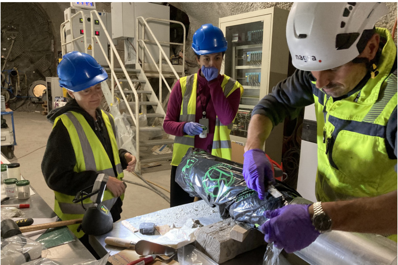
Figure 4: HE-E: Sampling from the overcored clay/bentonite interface (S. Schefer, swisstopo).
