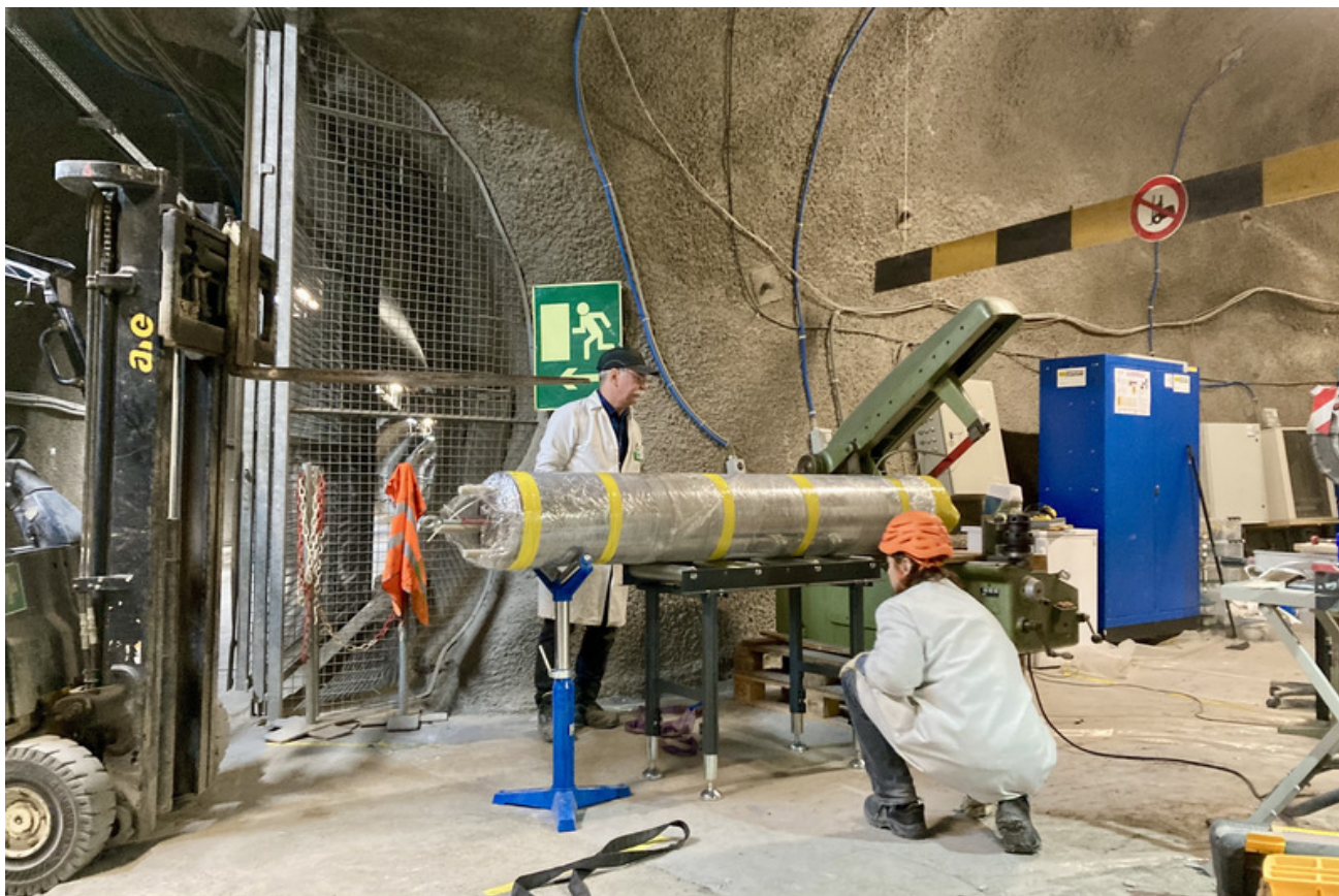
Figure 2: CI-D: The core is in place, ready for sawing. It weighs around 500 kg (S. Schefer, swisstopo).
