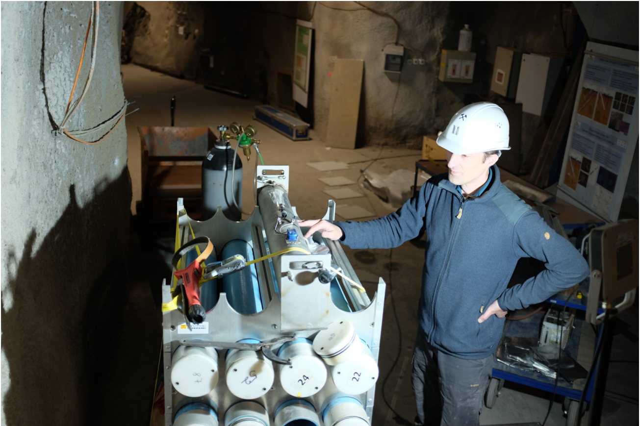
Figure 5: HE-F: The core section 6.22 - 7.16 m was stored after evacuation under nitrogen gas in a special liner with continuous logging of temperature, pressure and humidity. The liner allows gas sampling through a septum port (S. Schefer, swisstopo).
