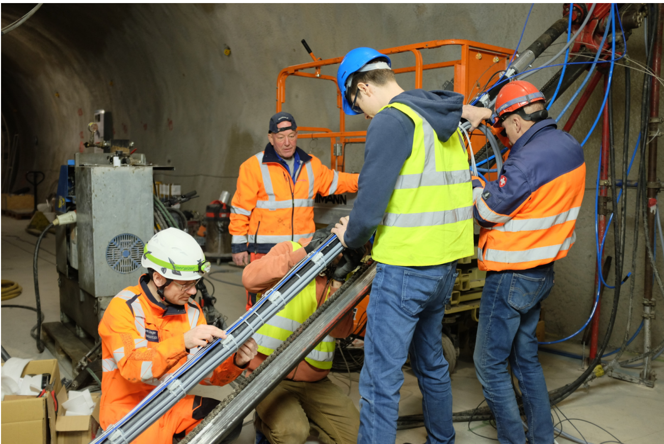
Figure 2: CL: Inserting the MMMS is a joint effort. There are many cables and lines to attach (S. Schefer, swisstopo).
