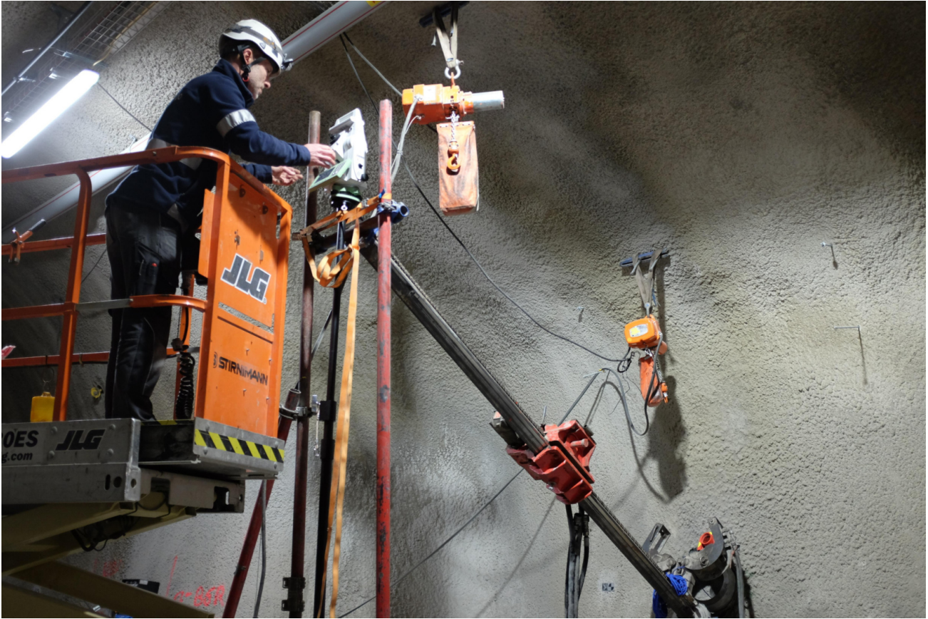
Figure 3: CL: Measuring the orientation of BCL-5 in a special setting (S. Schefer, swisstopo).
