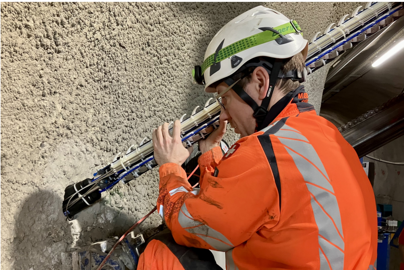
Figure 3: CL: M. Ziegler carefully pushing the MMMS into the borehole (R. Nicol, swisstopo).
