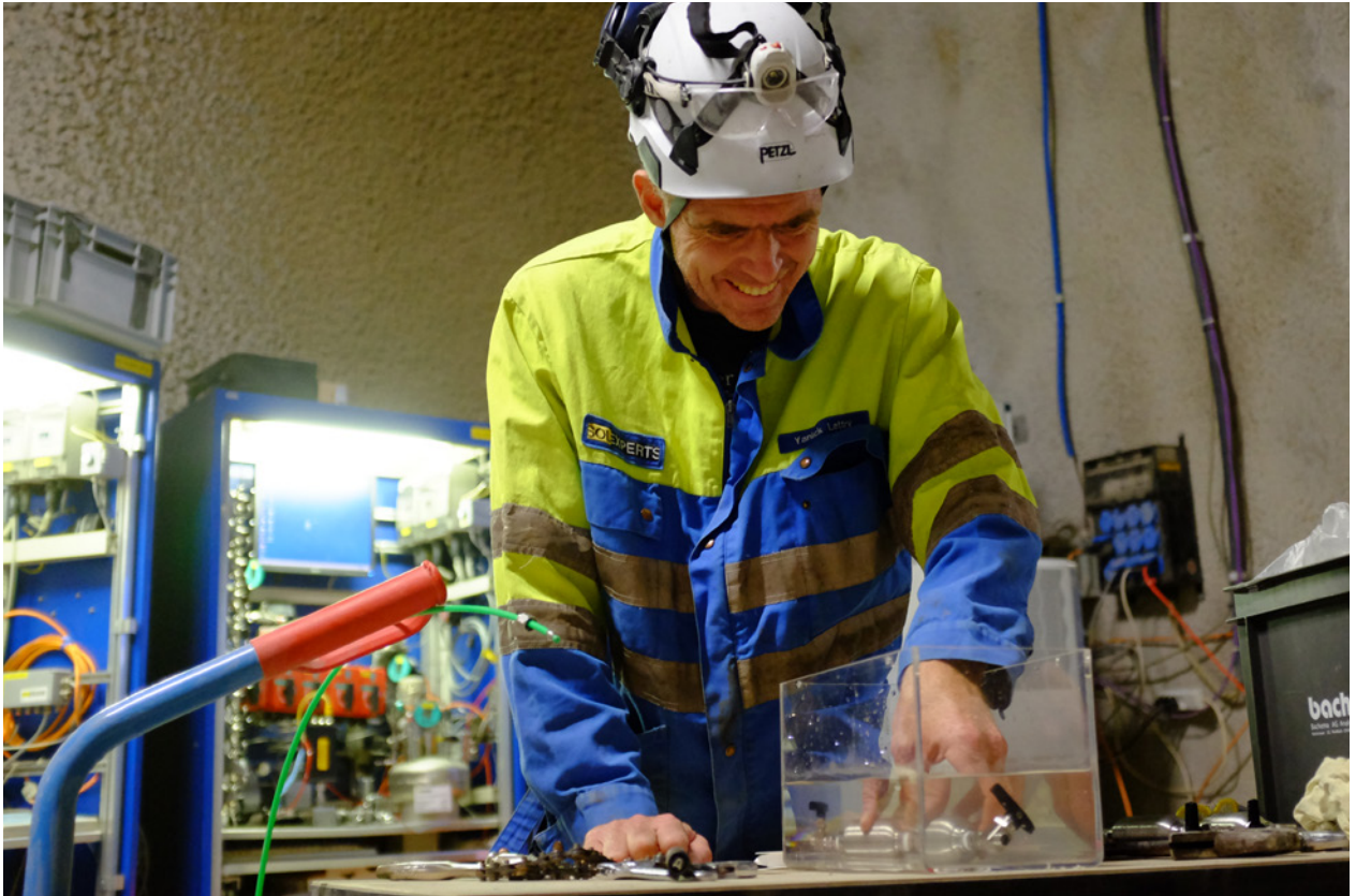
Figure 3: A technician checks the tightness of sampling containers at the site of the “Hydrogen Transfer” experiment.
