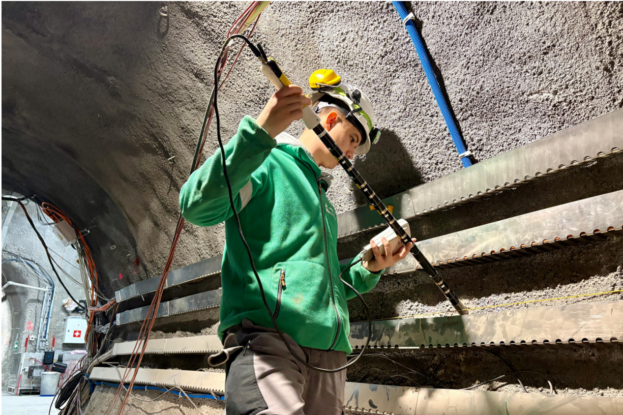
Figure 3: FE-M: Measuring the water content using the DeltaT profile probe. (J. Windisch, swisstopo)
