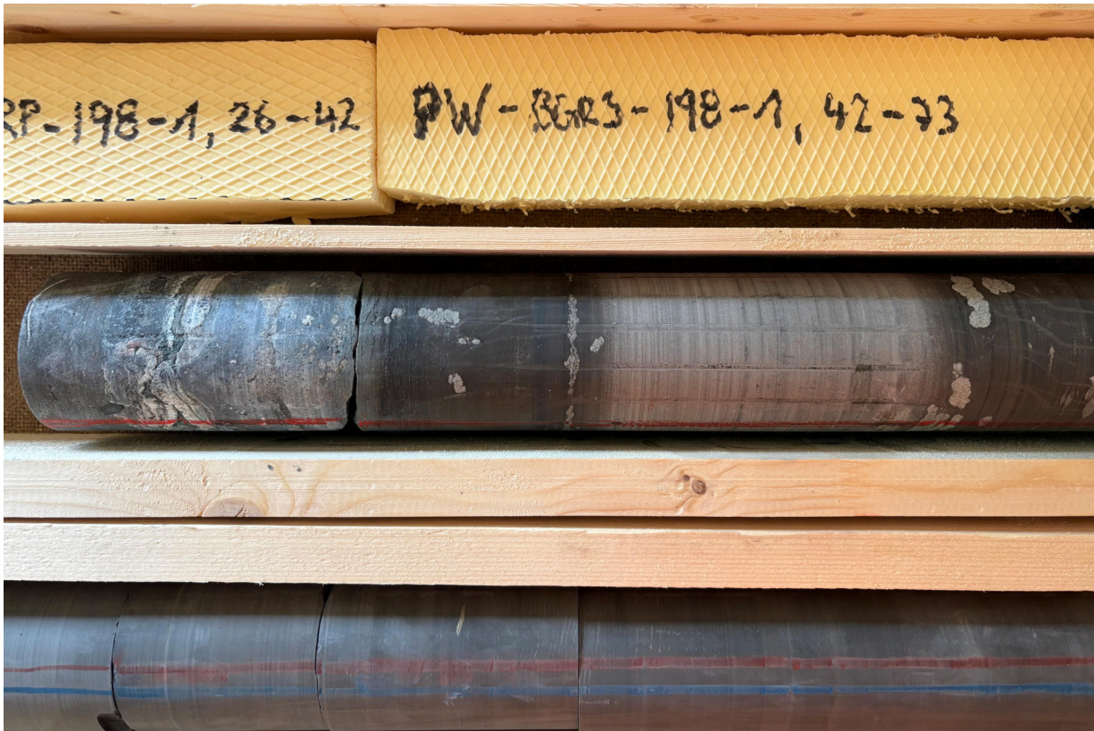
Figure 1: DB-B: Pyritic layers and a green bank marking the base of the Gross Wolf Mb. That's the last core run before cementing. (S. Schefer, swisstopo)
