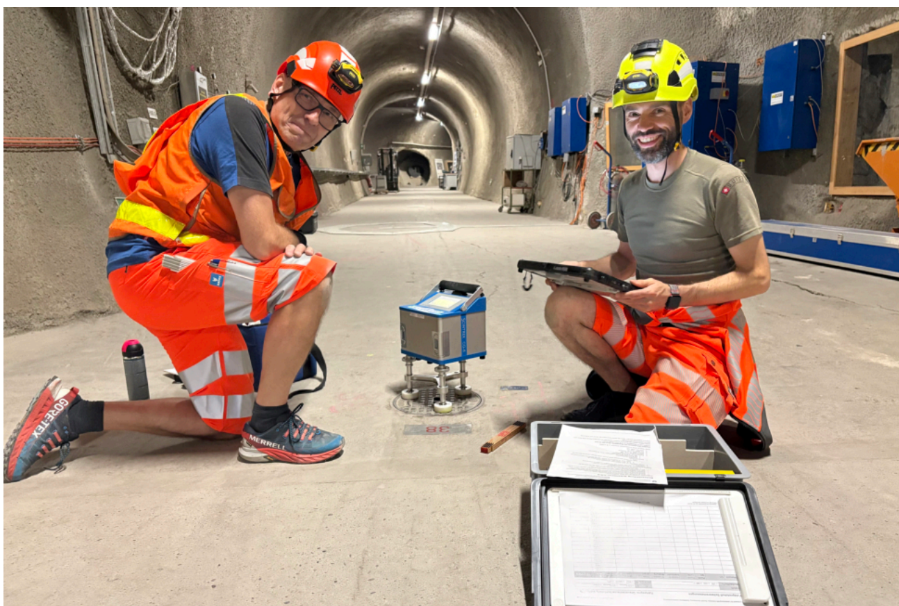
Figure 2: MH: Gravimetric measurements in Gallery 08 (J. Windisch, swisstopo)
