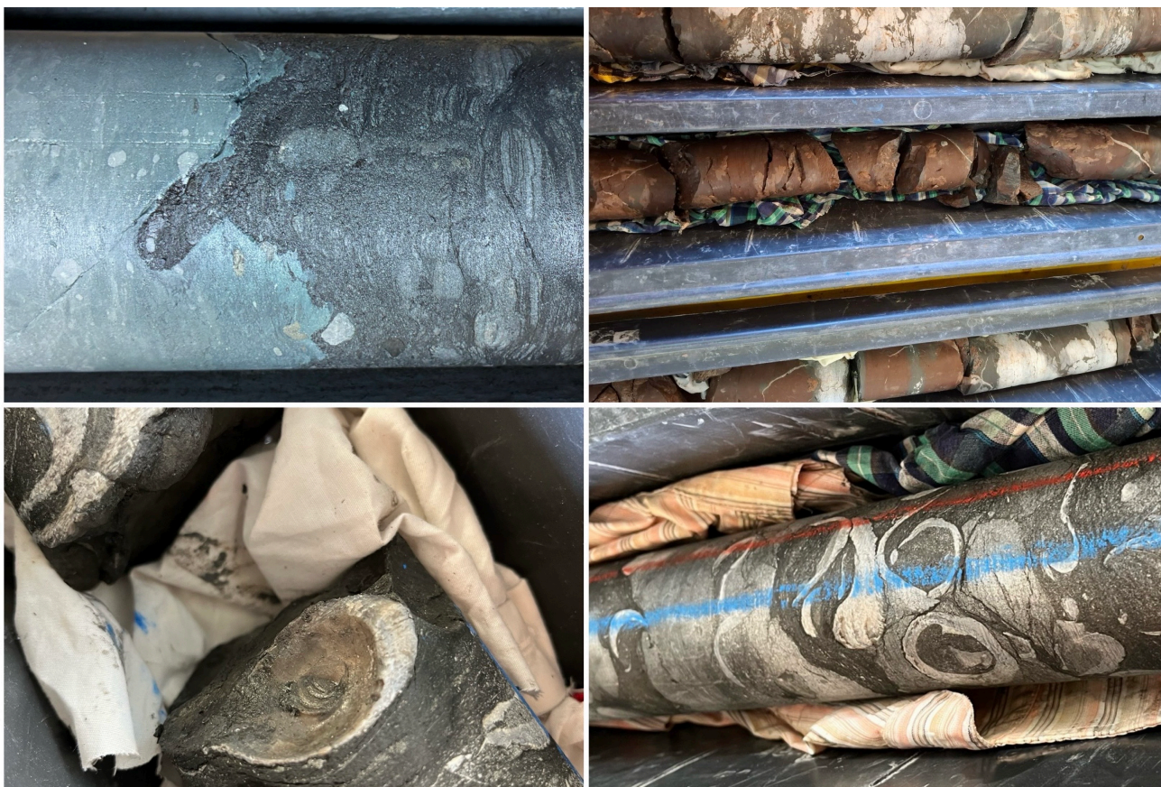
Figure 1: DB-B: Selection of core material: Klettgau Formation (top) and Beggingen Mb of the Stafflegg Formation (bottom) (S. Schefer, swisstopo)
