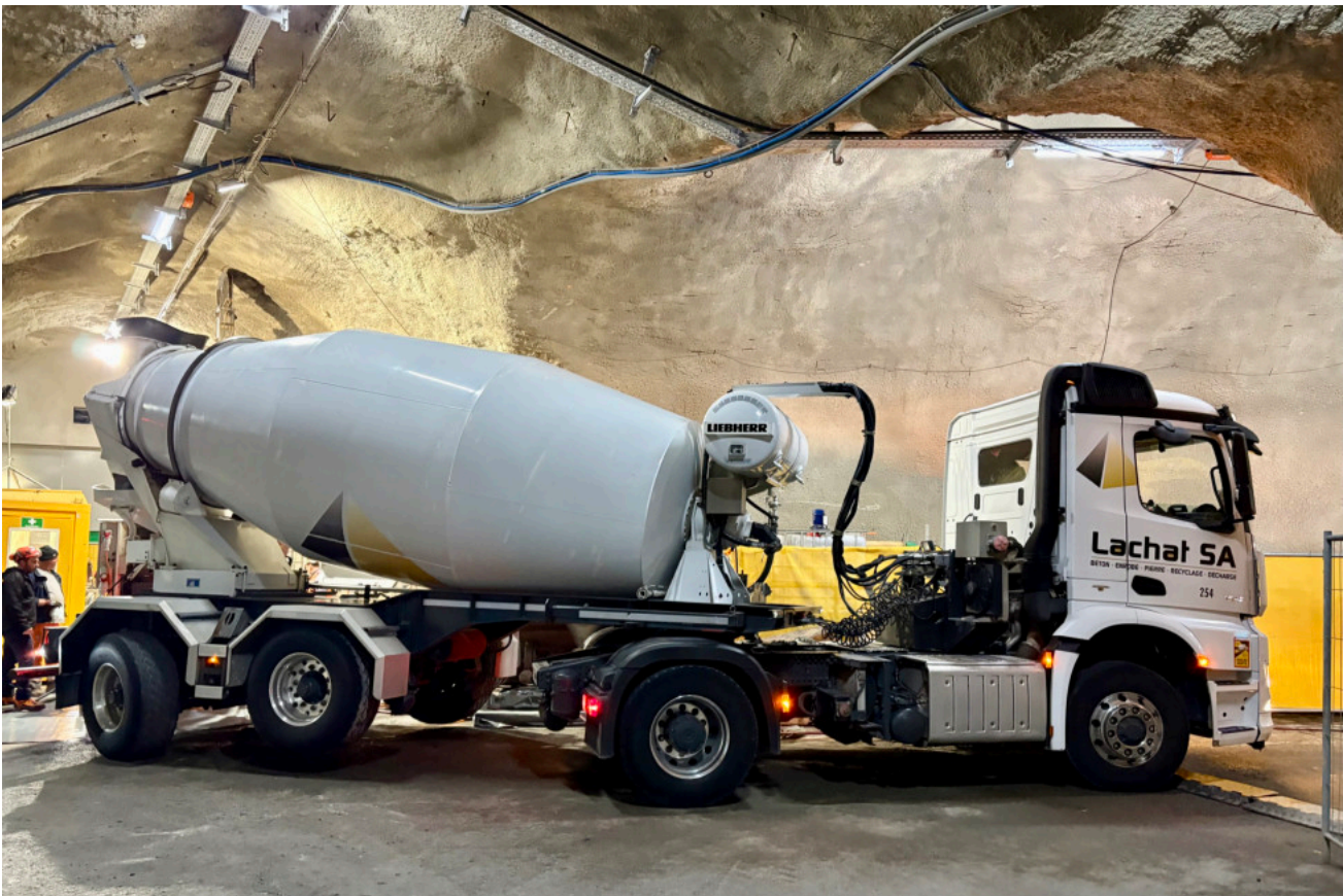
Figure 2: DB-B: Cementing the last section. (J. Windisch, swisstopo)
