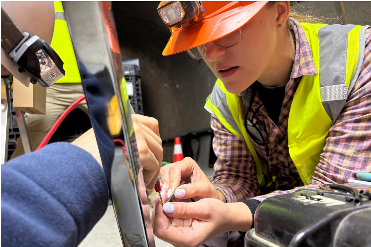
Figure 2: FS-B: Soldering the last connection for the piezoelectric measures (S. Schefer, swisstopo).
