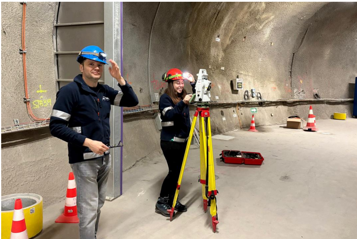
Figure 2: FS-B: Preparing the positioning for the geodetic measurements on the FS-B boreholes (S. Schefer, swisstopo).
