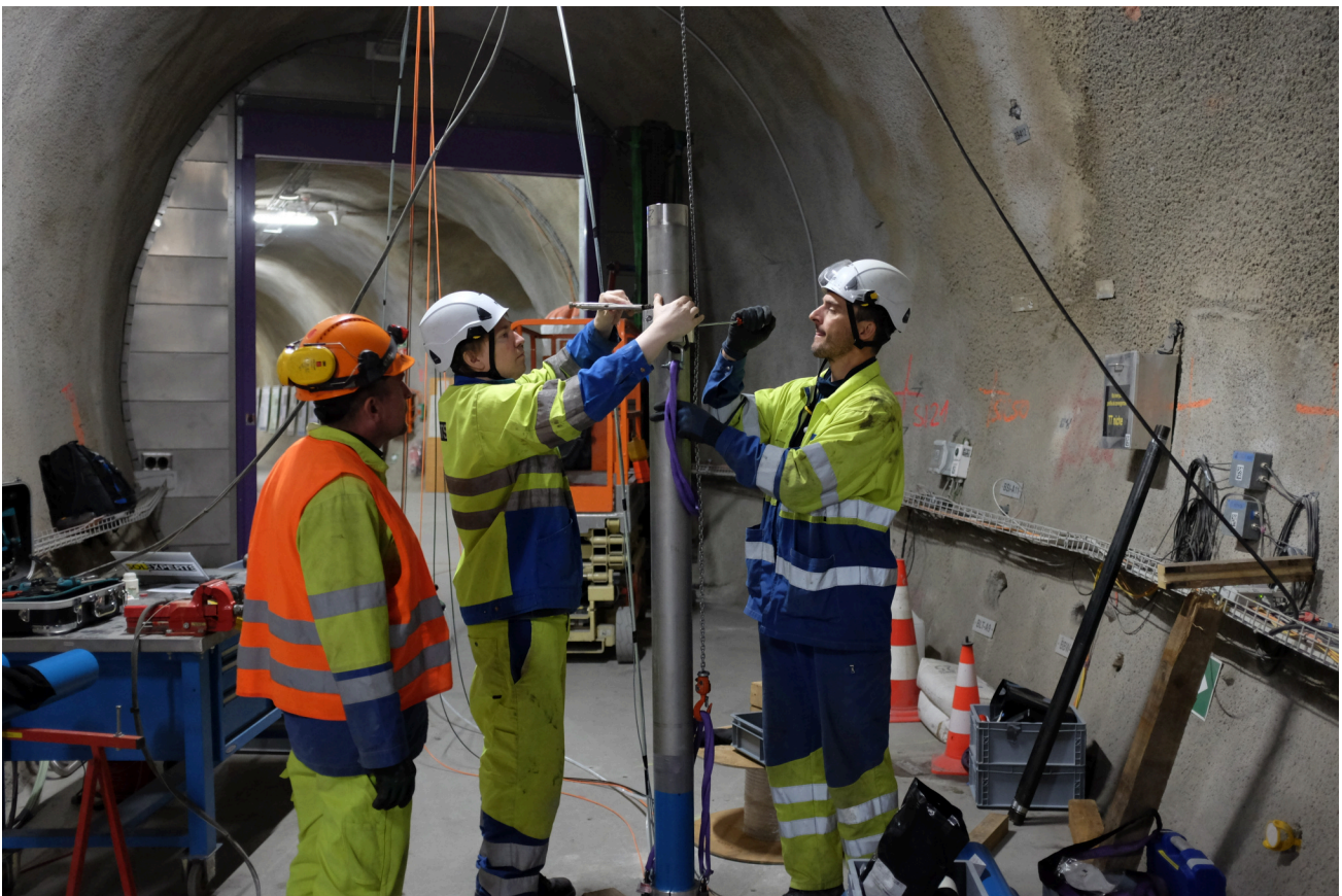
Figure 2: FS-B: Installing the fibres behind casing for BFS-B15 (S. Schefer, swisstopo).
