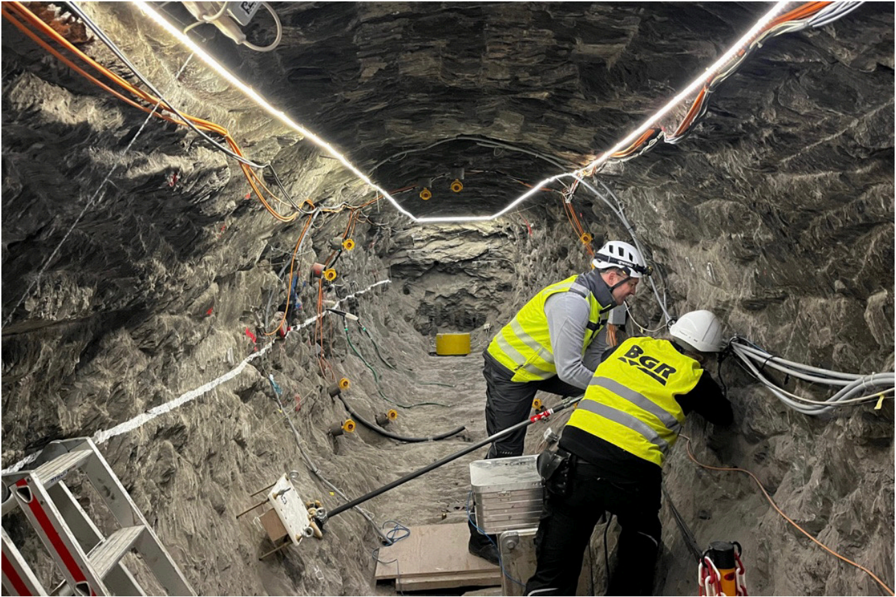
Figure 1: CD-A: S. Costabel and R. Dlugosch performing NMR measurement in Niche Open Twin (M. Abdelouhabi, swisstopo).
