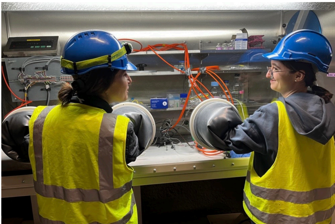
Figure 4: MA-A: Scientists from EPFL sampling microbial-rich pore water anoxically in the glovebox (M. Abdelouhabi, swisstopo).
