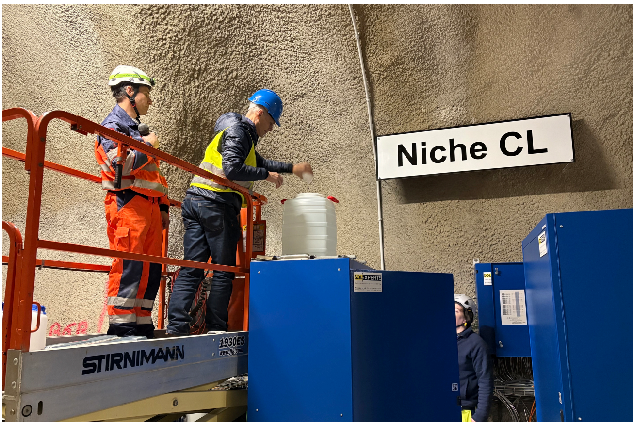
Figure 1: CL: Adding the tracer (2H and Br) to the tank (J. Windisch, swisstopo).
