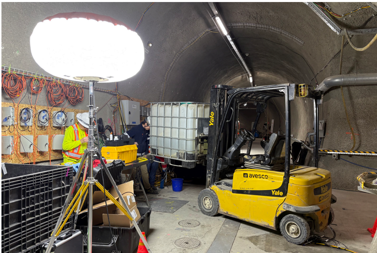
Figure 2: FS-B: 350 l of water are needed for a borehole of 78 m depth (S. Schefer, swisstopo).
