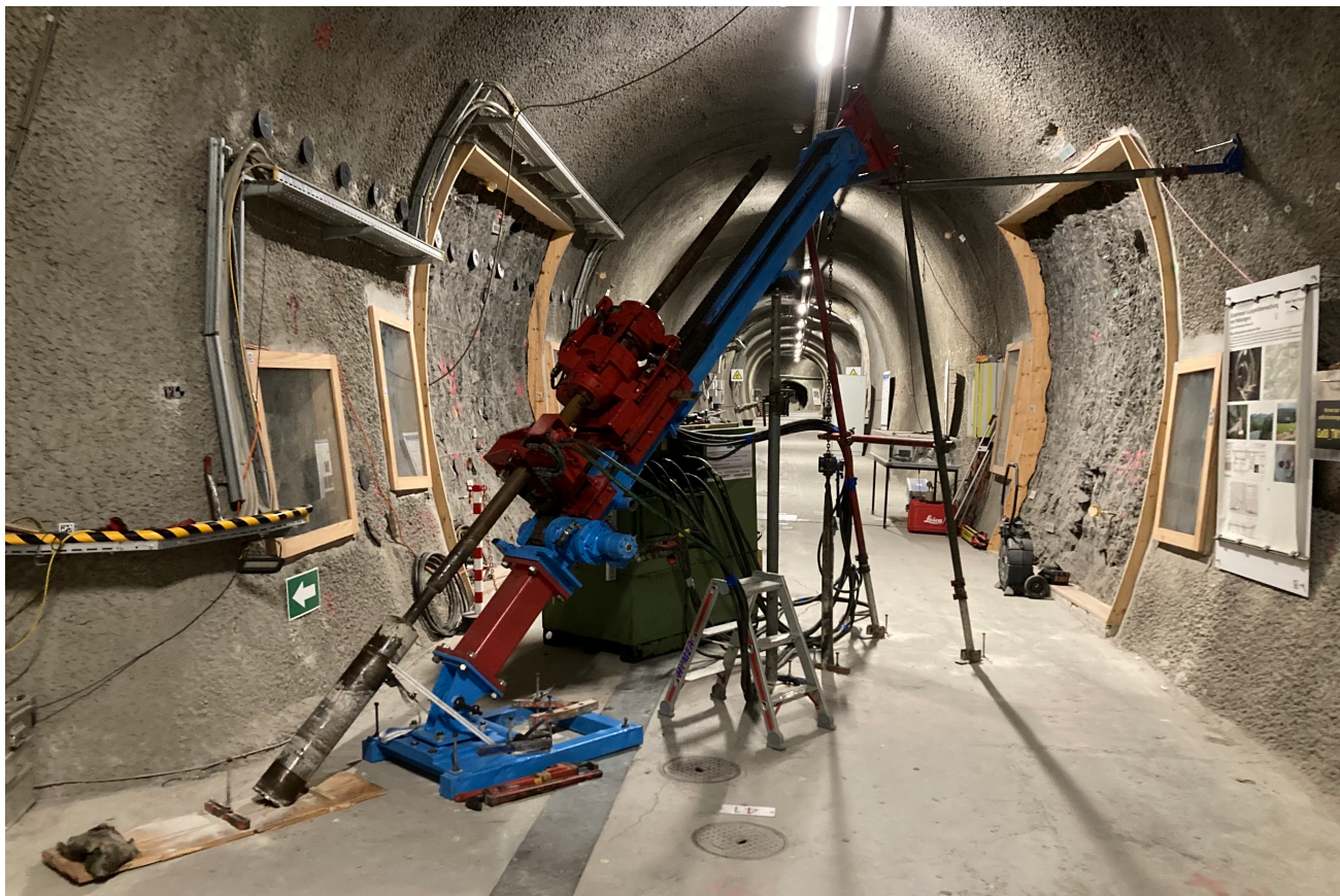
Figure 1: FS-B: Installed rig for BFS-B13 ready to start drilling next Monday (S. Schefer, swisstopo).
