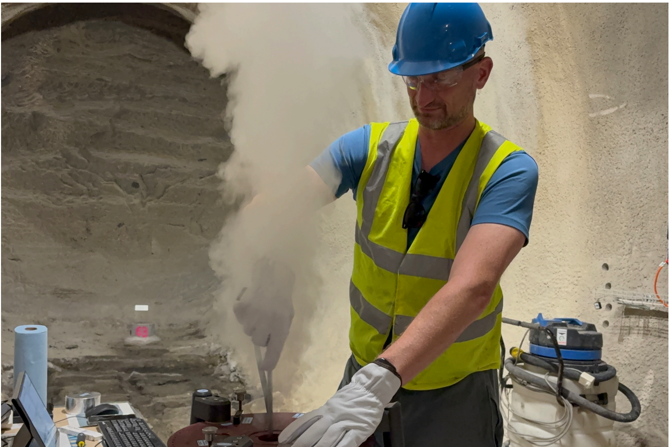
Figure 2: HS: Pouring warm helium inside the cooling chamber to defrost the interior (S. Schefer, swisstopo)
