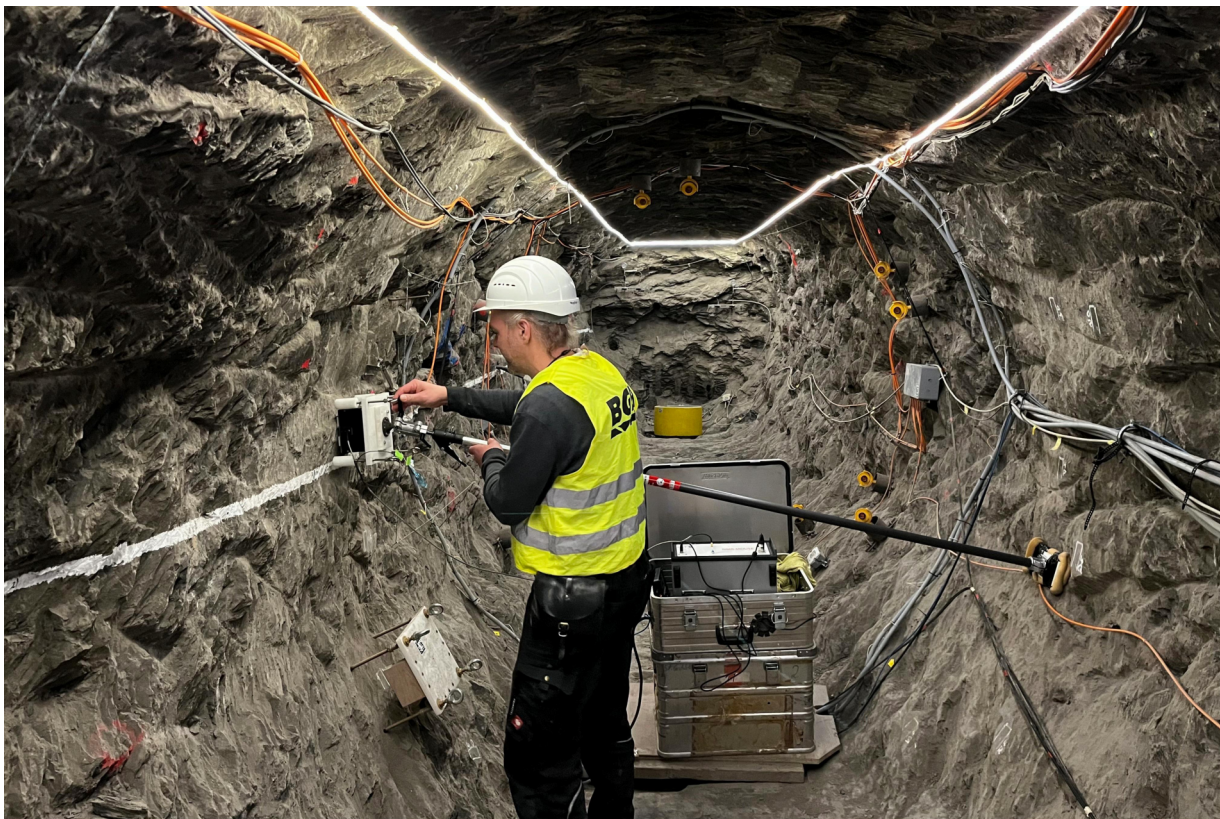
Figure 1: CD-A: Fixing the NMR mouse on the wall (S. Schefer, swisstopo).
