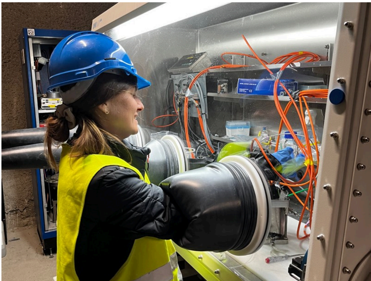
Figure 1: MA-A: C. Rolland (EPFL) removing the reactor out of the glovebox. Camille will do microbiological and chemical analyses on sand-bentonite incubated during 3 months (M. Abdelouhabi, swisstopo).
