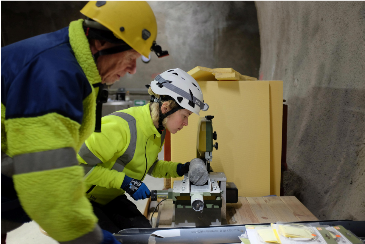
Figure 3: CL: Cutting smaller pieces for the gas analyses (S. Schefer, swisstopo).
