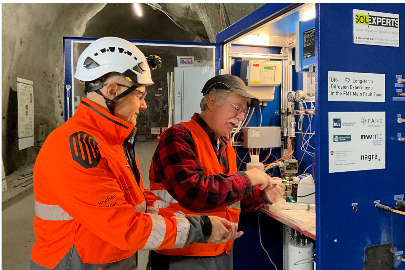
Figure 2: DR-E: pH calibration on DR-E2 (S. Schefer, swisstopo).
