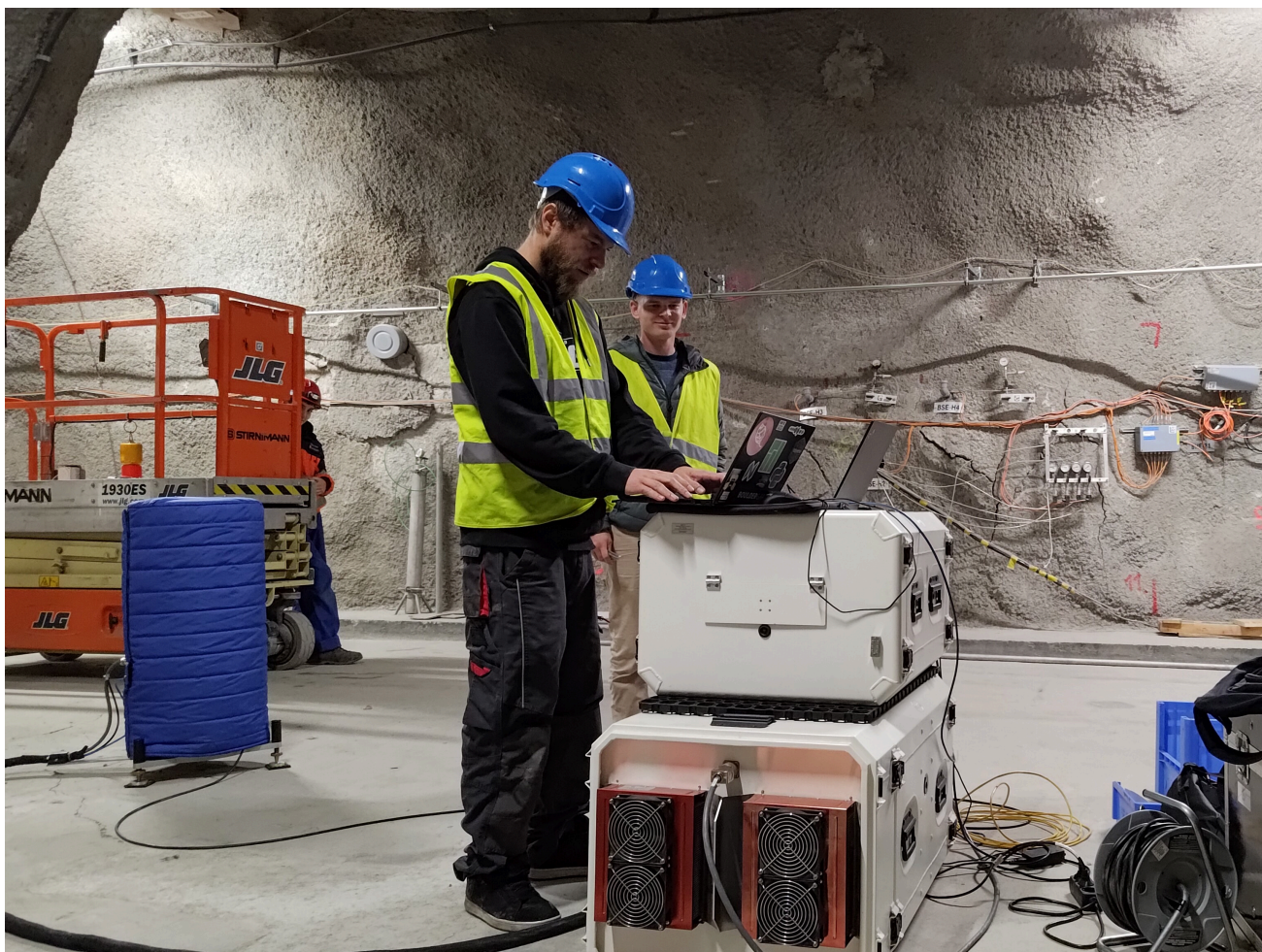
Figure 1: HS: Calibrating the gravimeter for the new measurements in Ga98 (M. Richard (swisstopo)).
