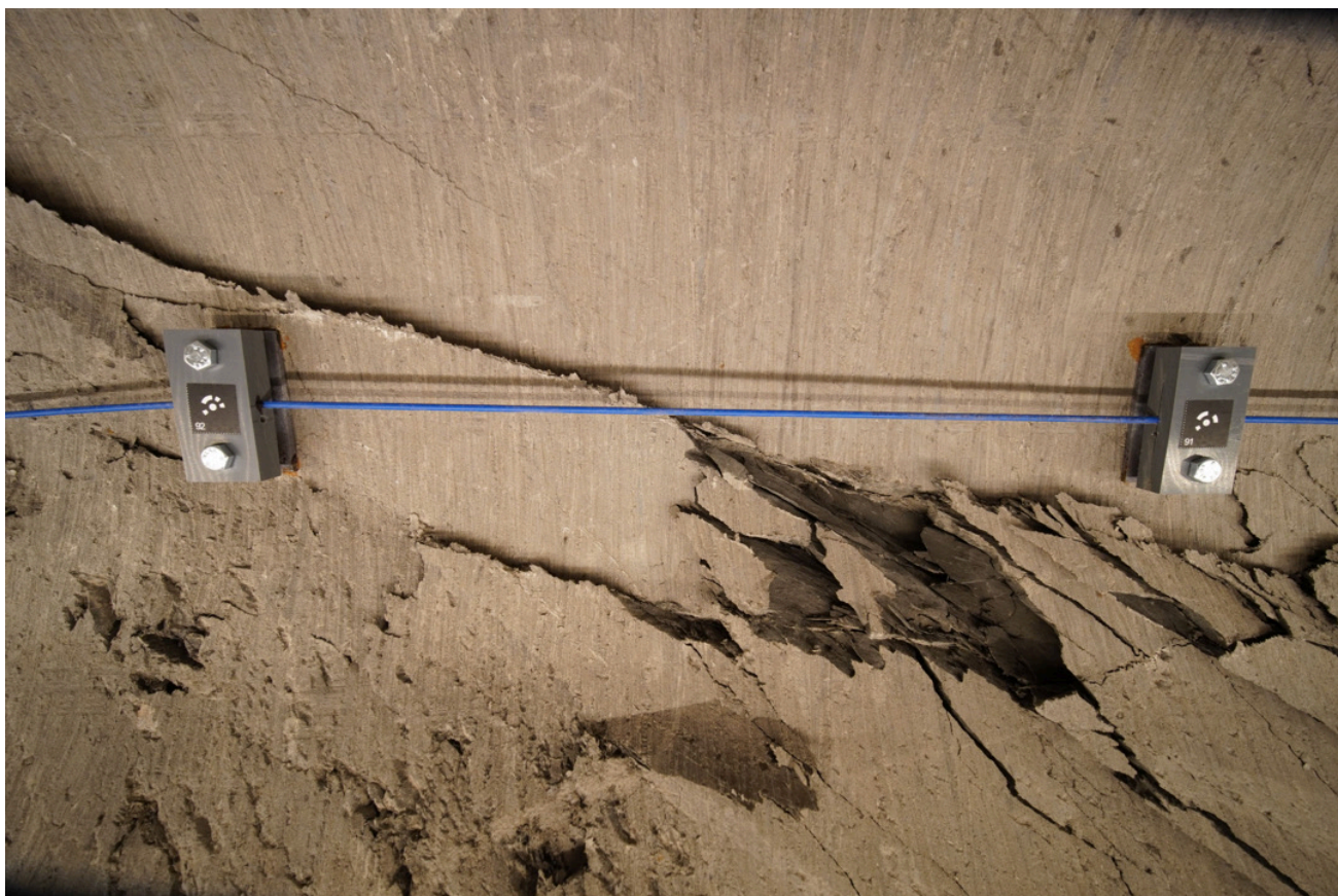
Figure 3: PF-A: 1 out of 6240 images taken with a 9 mm lens camera of the photogrammetric survey system inside the experiment borehole BPF-7. Image width is about 50 cm. The image shows a portion of the borehole wall with fixations (grey) of a FO-strain sensor cable (blue). These sensors and the photogrammetric 3D model produced from all 6240 images are used to assess the temporal and spatial evolution of borehole deformation and damage such as borehole radial convergence, displacement of discrete tectonic faults, borehole breakouts as well as induced cracks as seen in the image (M. Ziegler, swisstopo).
