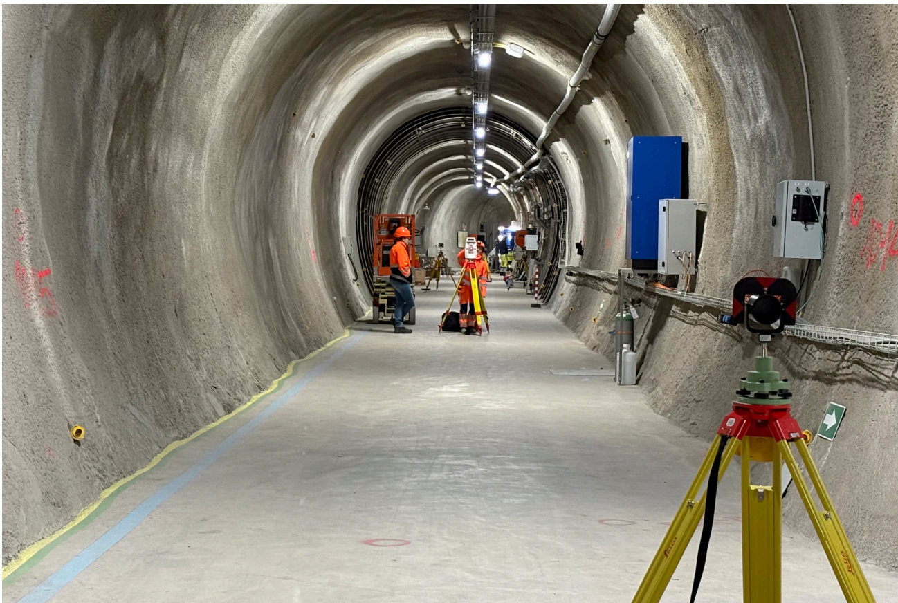
Figure 2: Mont Terri URL: Convergence measurements in Ga18 (S. Schefer, swisstopo).
