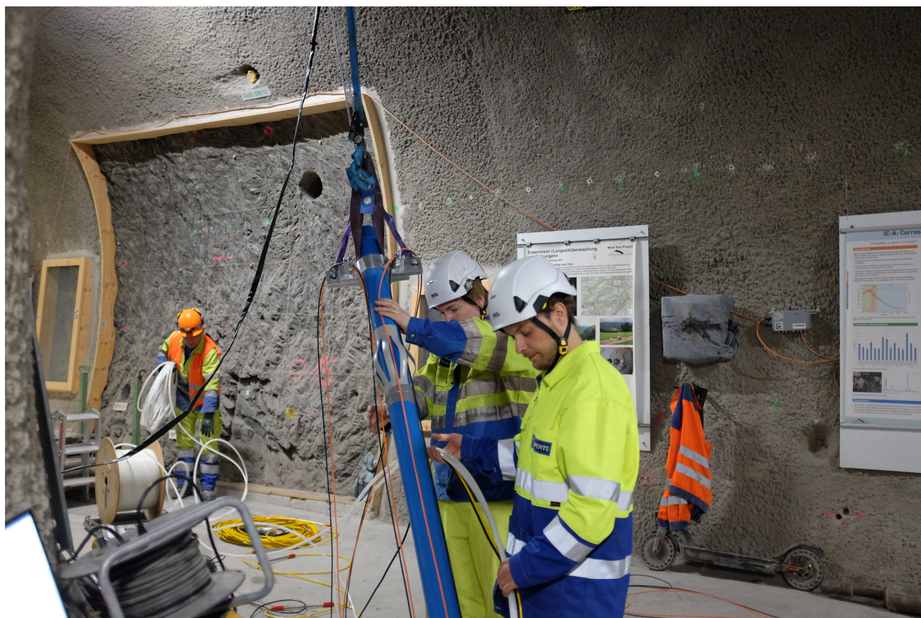
Figure 1: FS-B: Installation of the monitoring system into BFS-B13 (S. Schefer, swisstopo).
