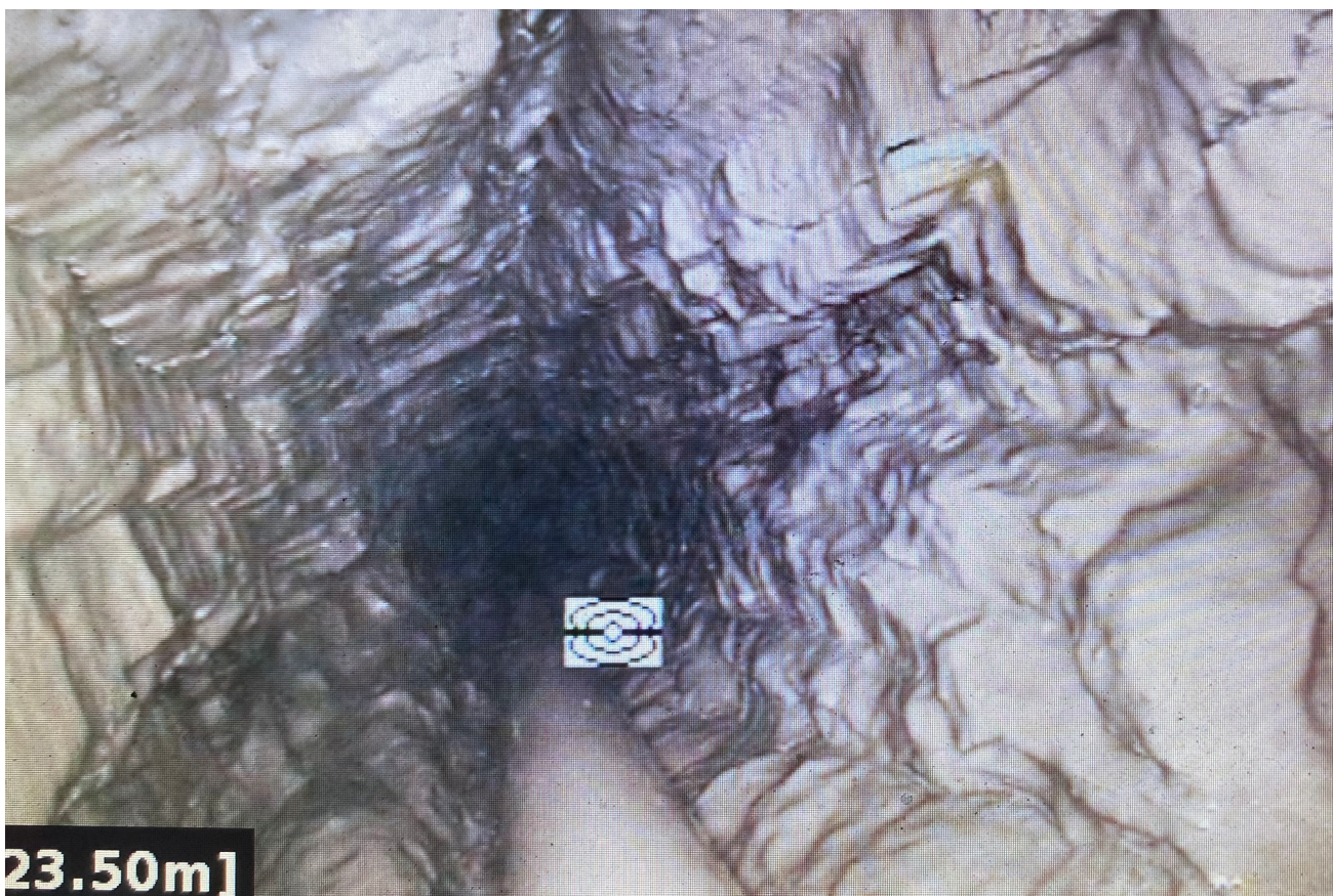
Figure 2: FS-B: The borehole is completely deformed with many breakouts (M. Ziegler, swisstopo).
