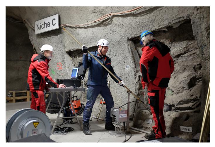
**Spotlight of the week:** C. Fixar, M. Kreutz and D. Novotny (BGR) tested a borehole laser scanner inside multiple boreholes. This tool produces a point cloud from the borehole allowing a very accurate survey of the surface inside the borehole. The picture shows the BGR-team in front of BSO-34 in the Niche C (Figure S. Schefer, swisstopo).
