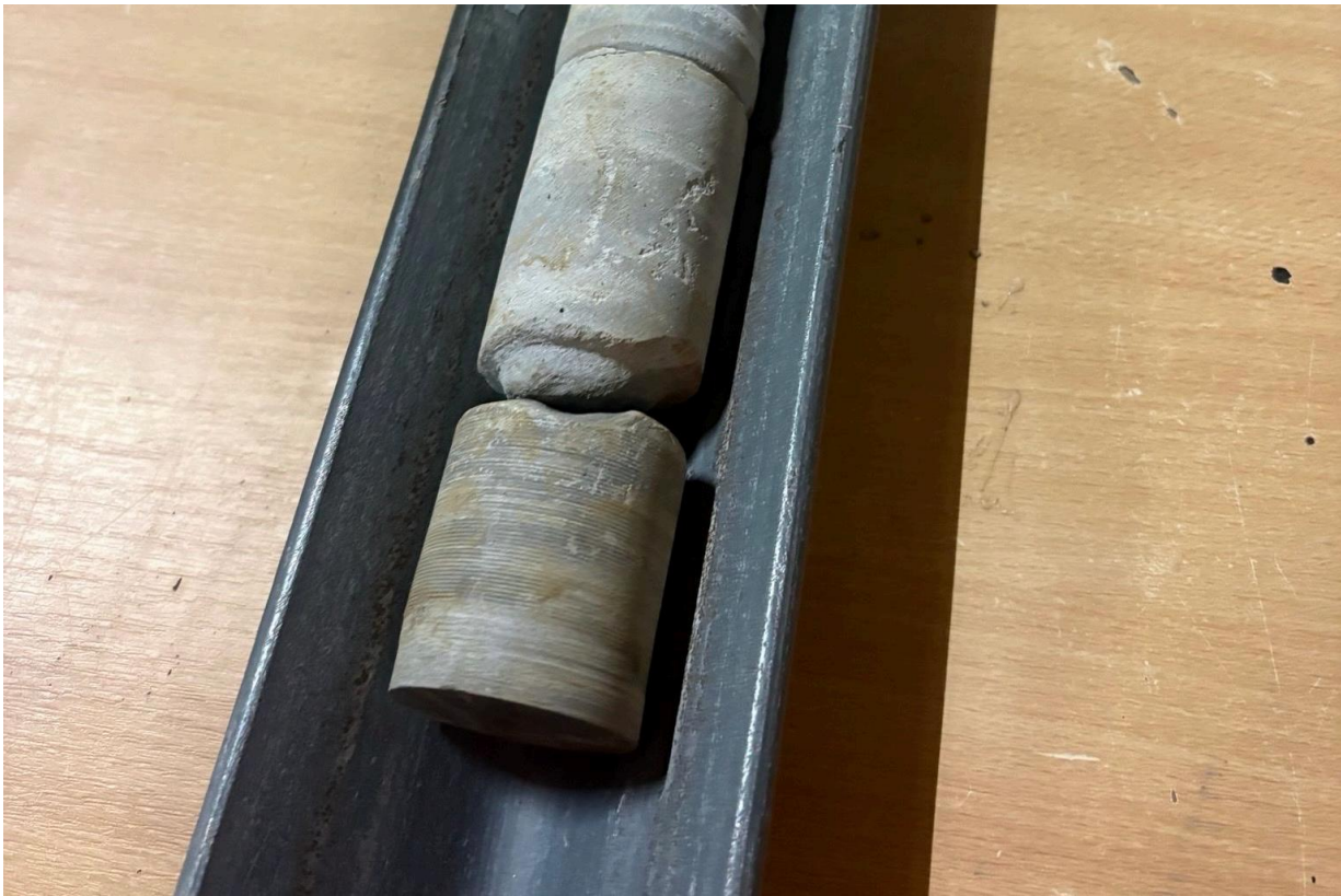
Figure 1: DB-B: Transition from cement to Schinznach Formation (S. Schefer, swisstopo)
