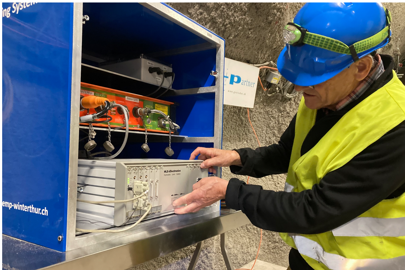
Figure 1: SM-C: E. Meier readjusting the HLS with the old and now repaired configuration (S. Schefer, swisstopo).
