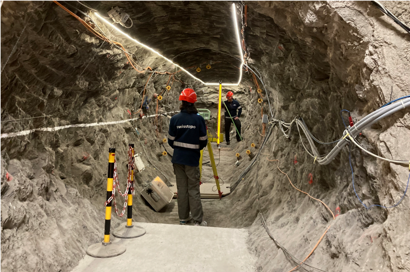
Figure 1: CD-A: Leveling in Niche Open Twin (S. Schefer, swisstopo).
