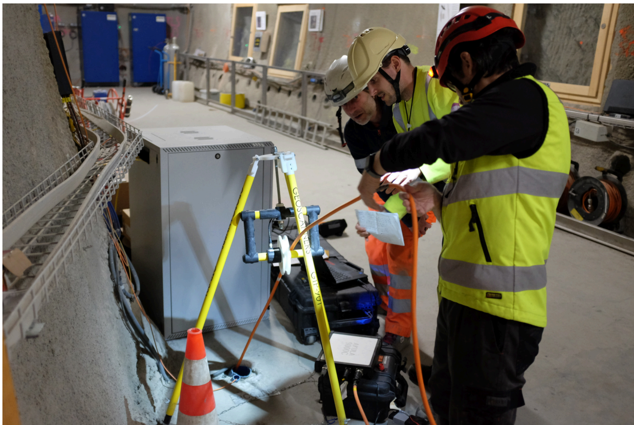
Figure 2: CS-E: Installing the GPR in BCS-D5 (M. Abdelouhabi, swisstopo).
