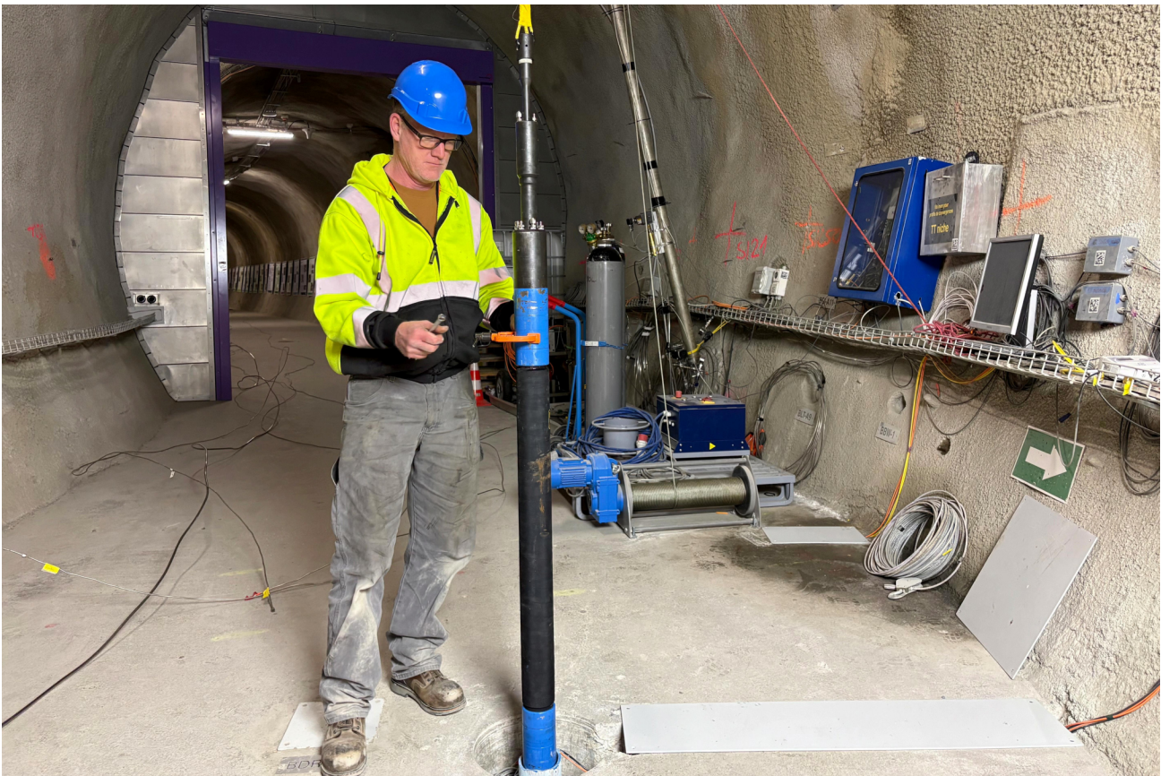
Figure 3: FS-B: Lowering the system into BFS-B15 is about to start (S. Schefer, swisstopo)
