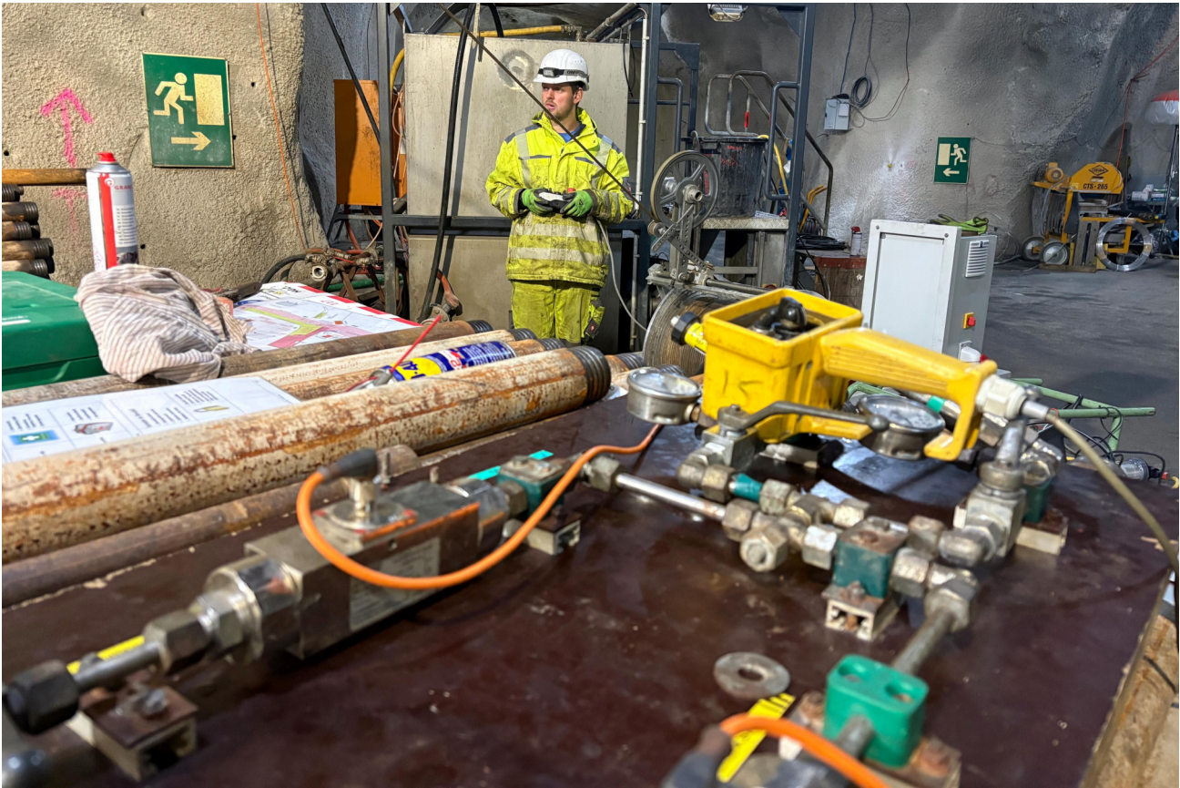
Figure 2: DB-B: The flow board for the sleeve reopening test (S. Schefer, swisstopo)
